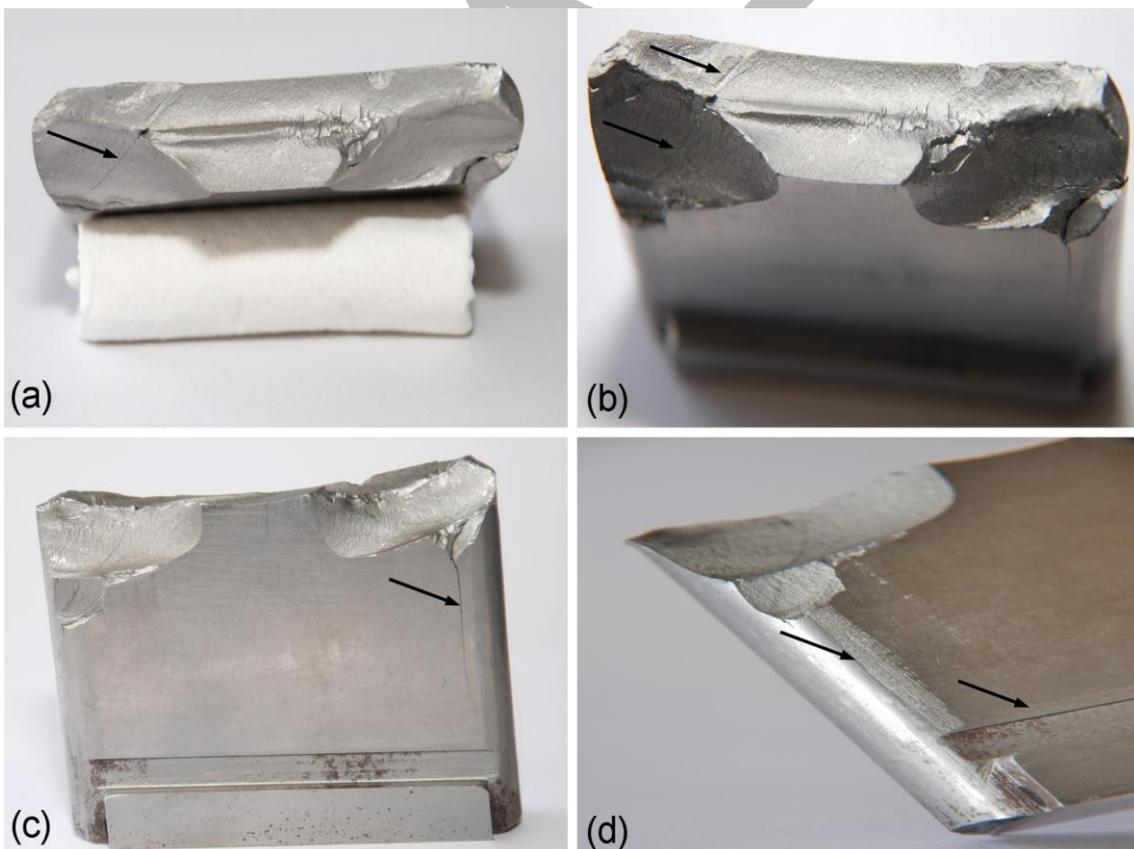
**Figure 5:** General aspects of the fragment of D1 cutting tool; (a) Fracture surface, (b) Striations on the fracture surface, (c) Secondary crack on the lateral surface, (d) Abrasion on the lateral surface of the tool.
