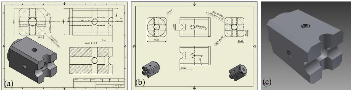
**Figure 9:** (a) Projection of the dimensional measurements, (b) Projection of the dimensional measurements (manufacturing details), (c) Moving blade: three dimensional presentation (3D).
