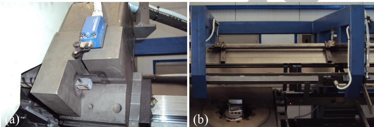
**Figure 2:** Machine detail; (a) Cutting die placed at the exit of the alignment chamber, (b) Forming die.
