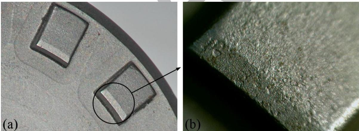
**Figure 7:** Detail of the seating on the teeth: a) General view, b) Taper on the inner edge of the teeth.
