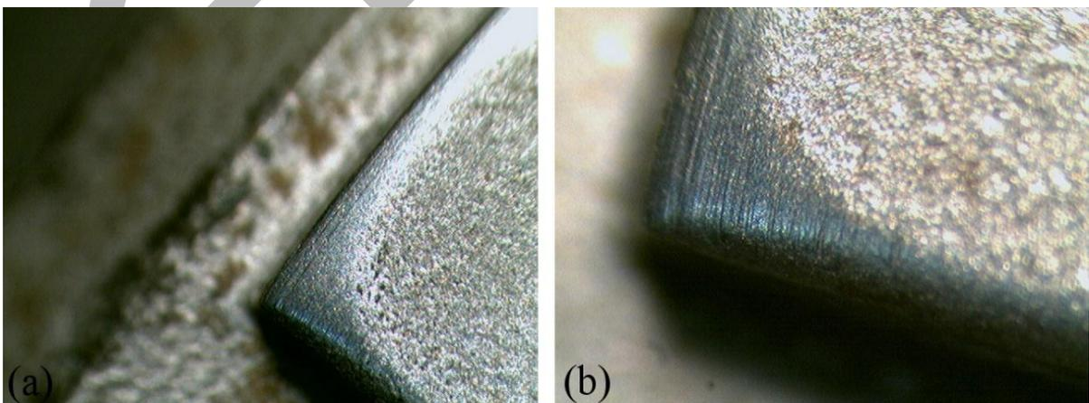
**Figure 5:** Teeth detail; (a) Radius due to erosion on the edge, (b) Microwelding zone.
