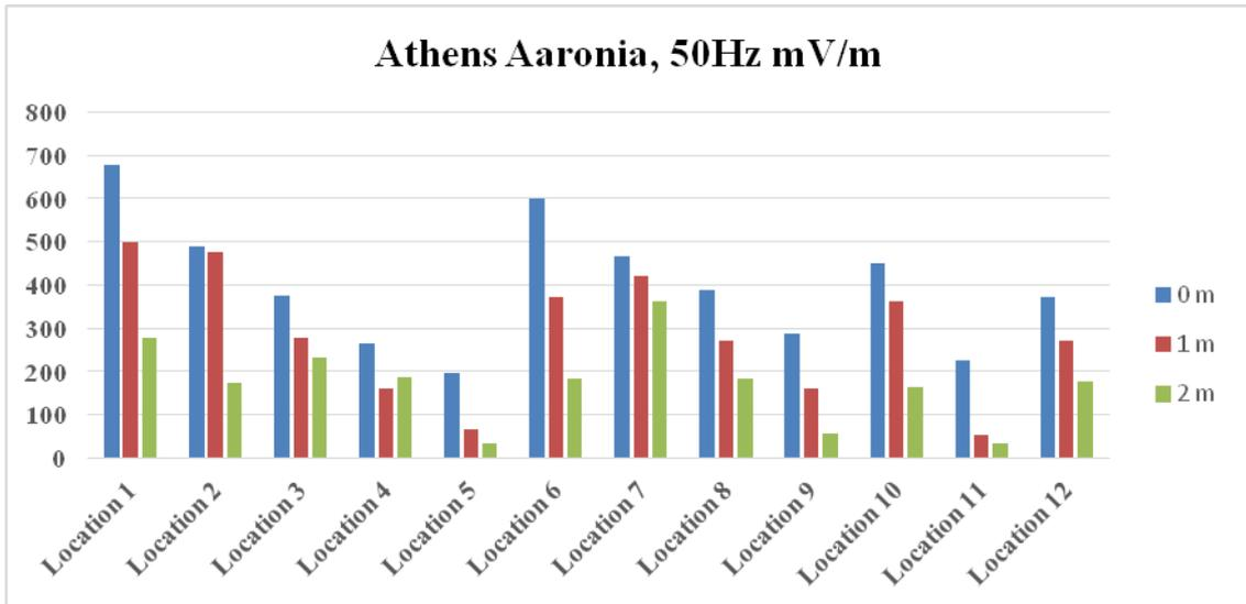
Fig.6 Aaronia measurements, 50Hz mV/m in Athens
