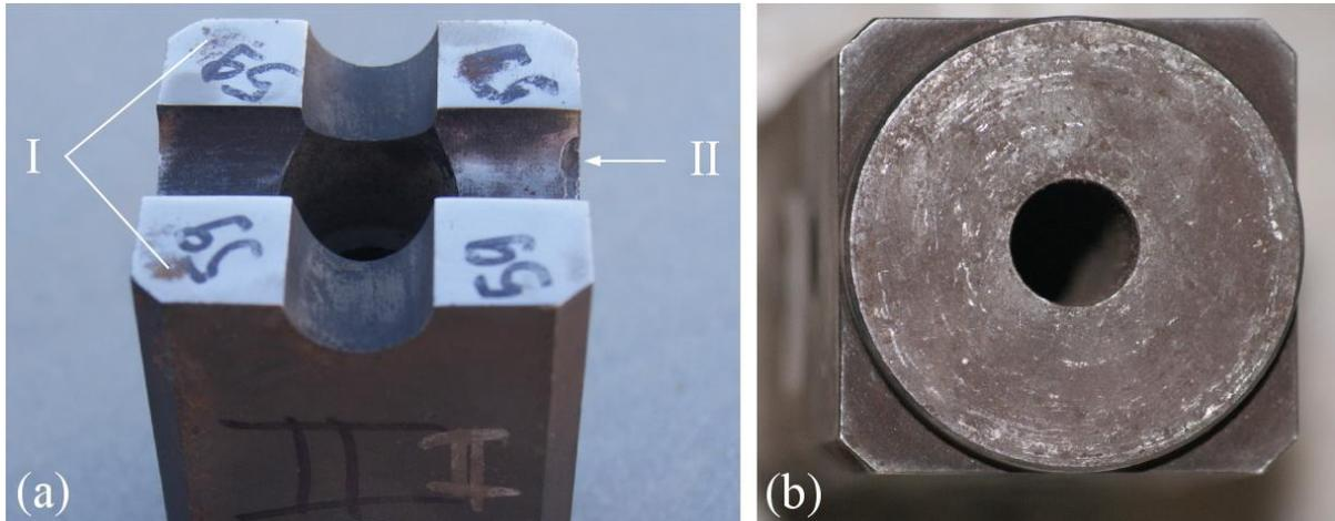
**Figure 5:** Detail of the moving blade: a) Working surface b) Opposite side.
