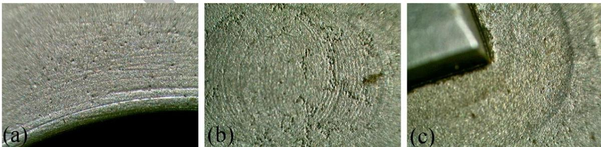
**Figure 3:** Detail of the working surface; (a) Pores, Mx20, (b) zone with rough surface finishing, Mx20 (c) Fingerprints around an unfractured tooth, Mx20.
