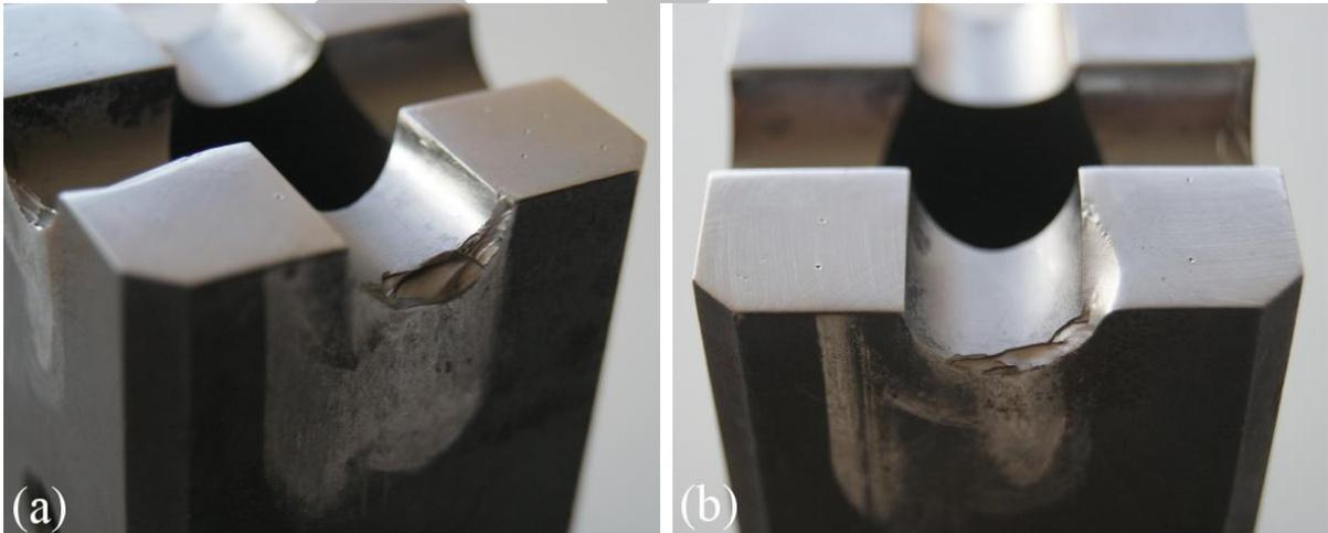
**Figure 8:** Detail of the dies; fracture of the cutting edges: (a) Piece I, (b) Piece II.
