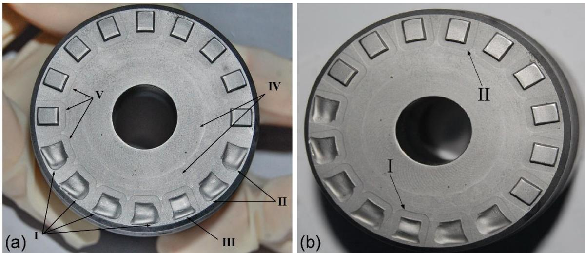
**Figure 2:** (a) General aspect of the working surface after cleaning, (b) Fingerprints around the teeth.
