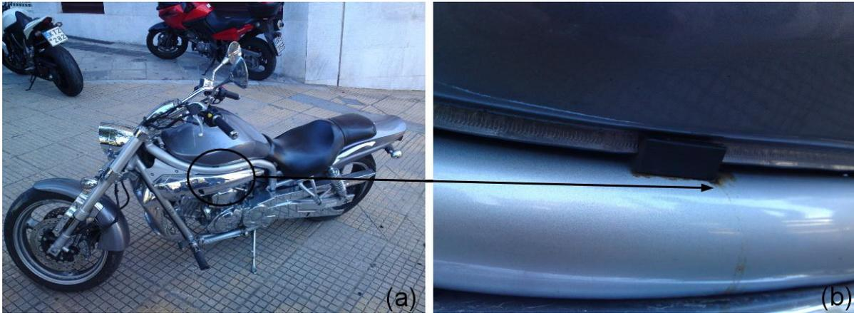
**Figure 1:** (a) General aspect of the motorbike, (b) Point of the fuel leakage.
