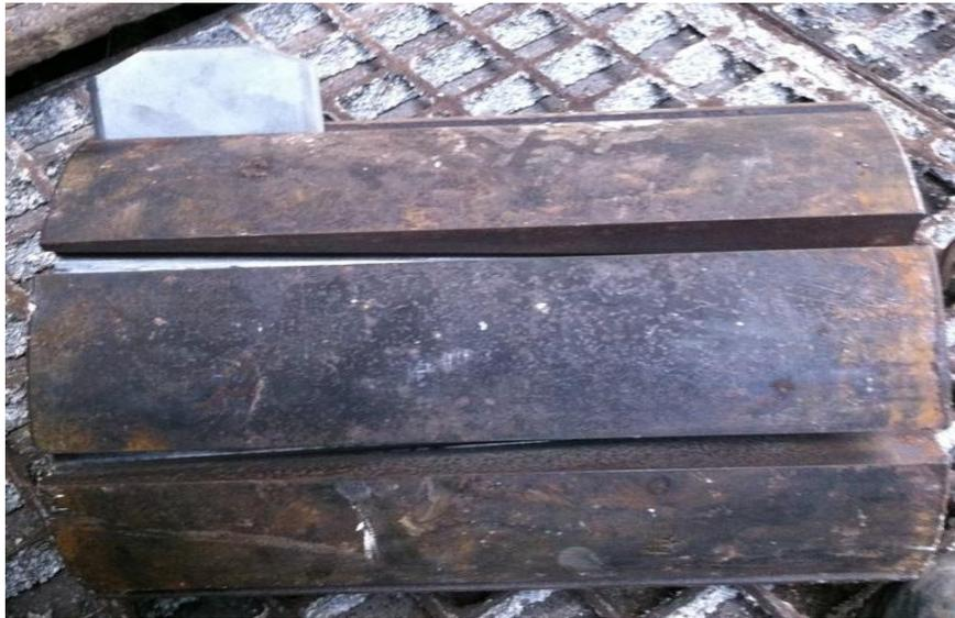
**Figure 2:** The assembly of cutting tool on internal cylindrical forming dies.
