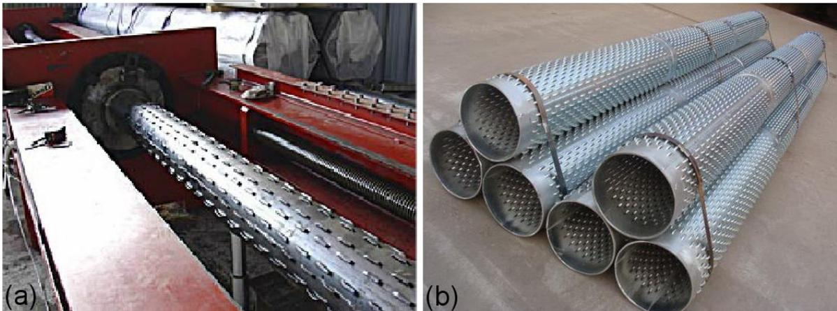
**Figure 1:** (a) Bridge slot forming machine, (b) Bridge slot filter pipes.
