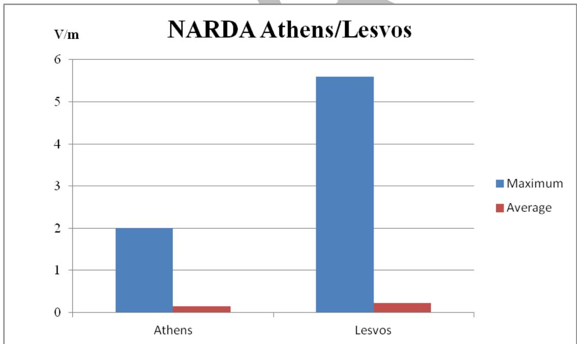
**Fig.13** NARDA measurements electric field compared
