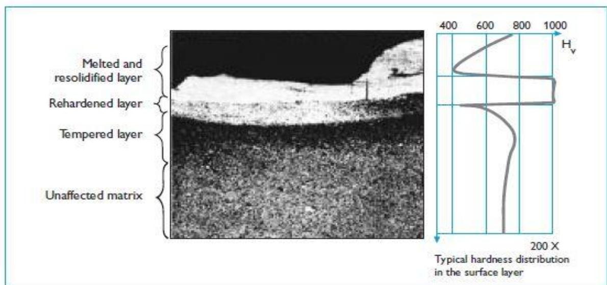
**Figure 4:** The heat affected zone after EDM machining [9]
