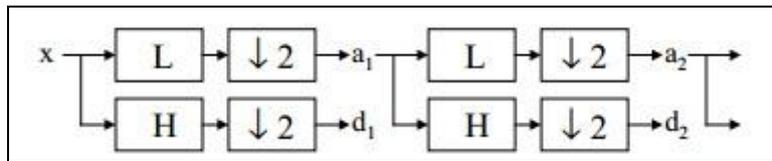
Figure 2. Discrete Wavelet Transform tree diagram.
