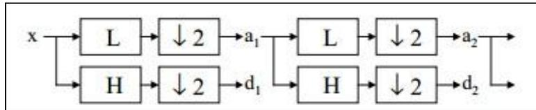
**Figure 2.** Discrete Wavelet Transform tree diagram.
