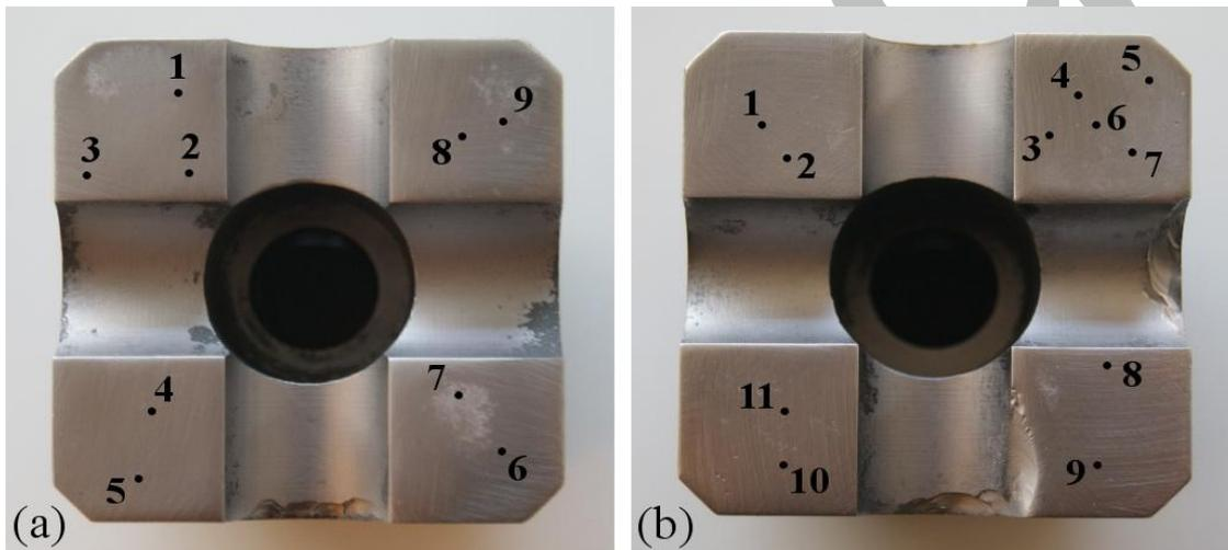
**Figure 10:** Hardness measurements points on the working surface; (a) Piece I, (b) Piece II.
