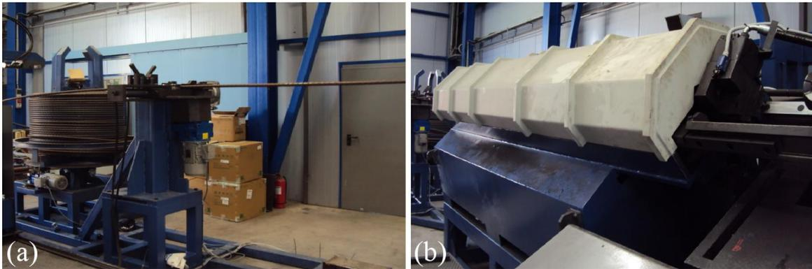
**Figure 1:** (a) Roll of raw material, (b) Machine detail: chamber of material alignment.
