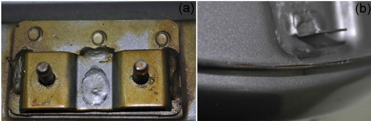
**Figure 6:** Fuel tank details; (a) Welding points on the failure area (b) Cracks on the circumferential seam welding line.
