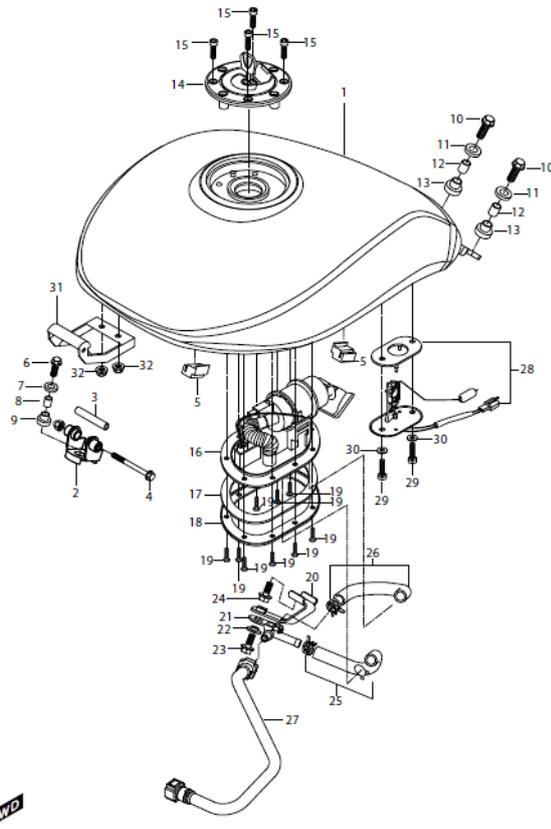
**Figure 2:** Assembly drawing of the fuel tank [11].
