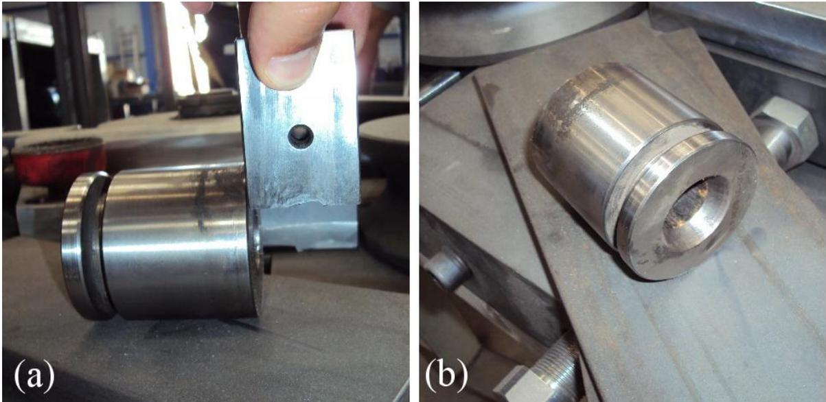
**Figure 3:** (a) General aspect of the cutting die, (b) The stable blade of the cutting die. The moving blade is placed in series with the stable one (Fig. 4). During cutting, it is pressed via a hydraulic system perpendicular to the bar axis, provoking shearing stresses as co acts with the stable blade. The side surfaces of the two parts are tangent during cutting.
