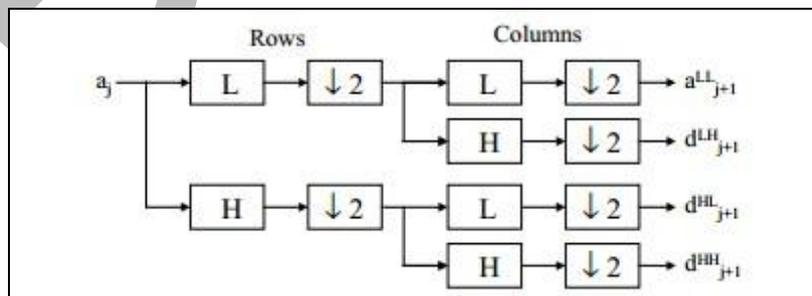
Figure 3. Wavelet decomposition of two dimensional pictures.
