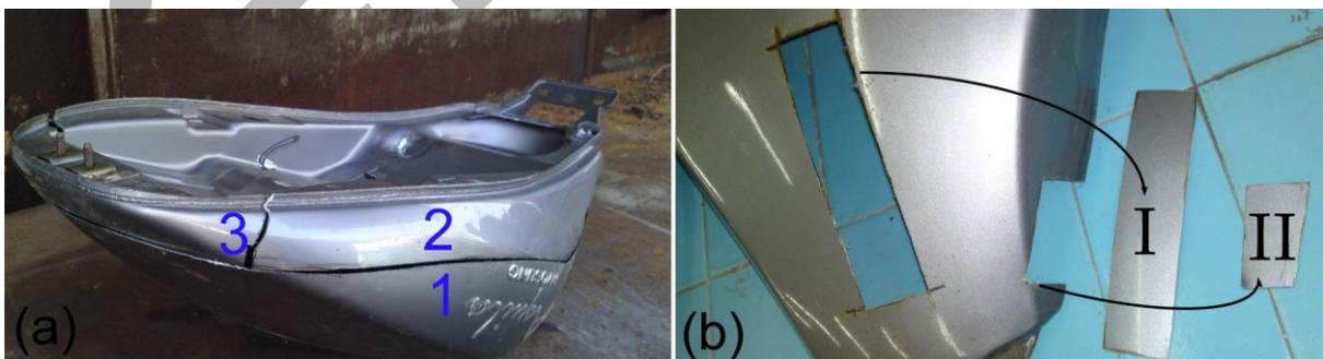
**Figure 6:** (a) First fuel tank fragmentation, (b) Sample selection from the first fragment; I-sample for chemical analysis, II- sample for hardness measurements.
