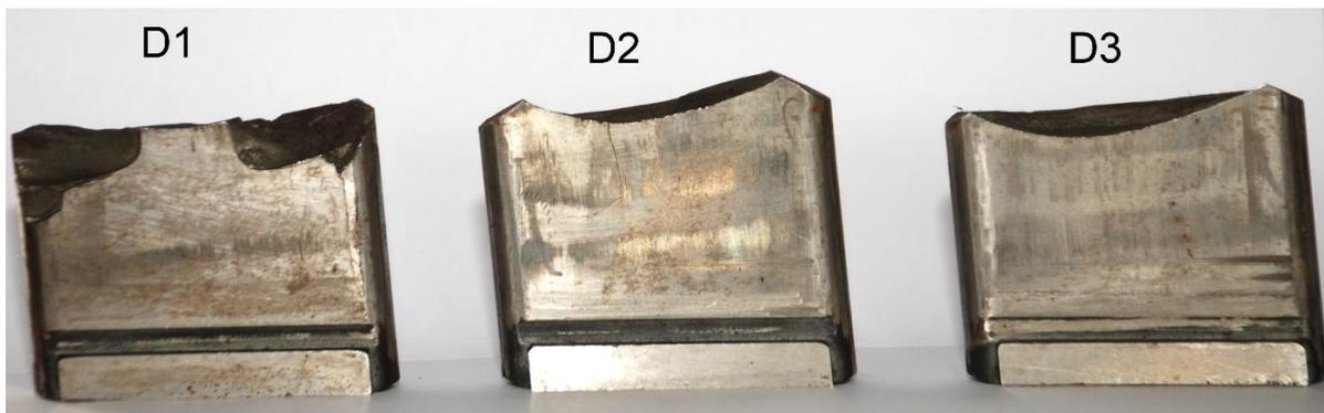
**Figure 4:** The fragment of the three failed cutting tools.
