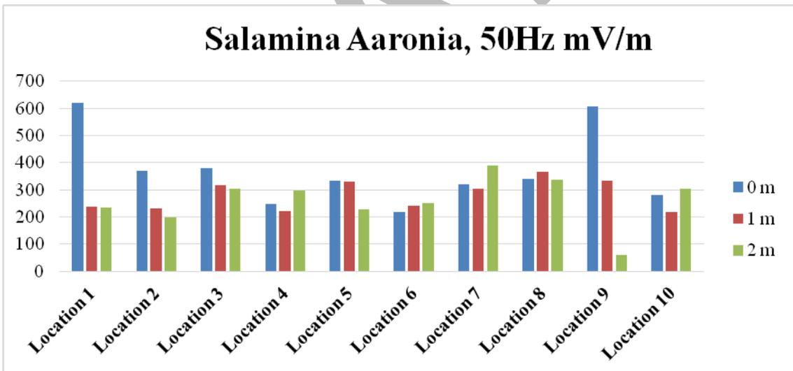
Fig.7 Aaronia measurements, 50Hz mV/m in Salamina
