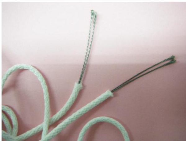
Woven lanyard with core consisting of yarns include metal strands, close view.
